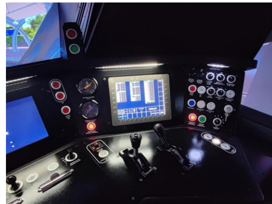
Fig 2: Photo of a fragment of the driver's desk of the SimFactor railway vehicle simulator located at the headquarters of Koleje Śląskie Company, together with a touch screen
