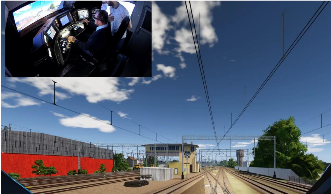
Fig 5: A driver in the driver's cabin of a railway vehicle simulator while conducting a test using eye-tracking glasses
