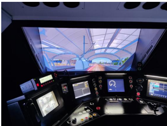
Fig 1: Photo of the driver's cabin of the SIMFactor railway vehicle simulator located at the headquarters of Koleje Śląskie
