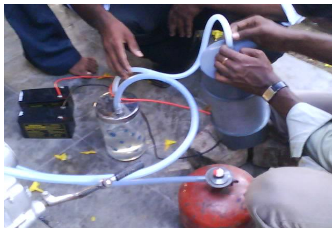
Fig 4.4: schematic views of Hydrogen tank, gas cylinder and battery (Two wheeler)
