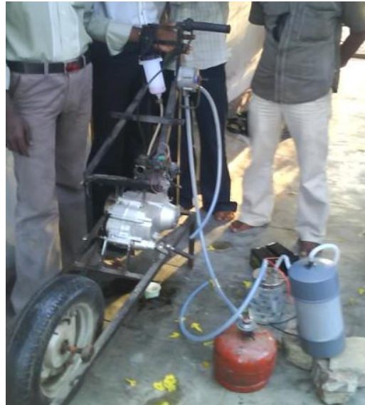
Fig 4.3: Schematic view of Hydrogen engine (Two wheeler)
