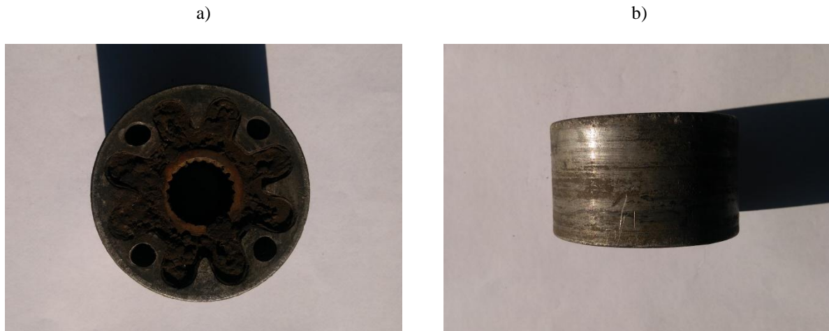
Fig. 2 Axis surface wear, a)side view, b) overview
